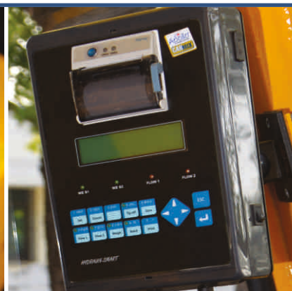
Electronic weighing system cum printer to get quality concrete as per mix design.
